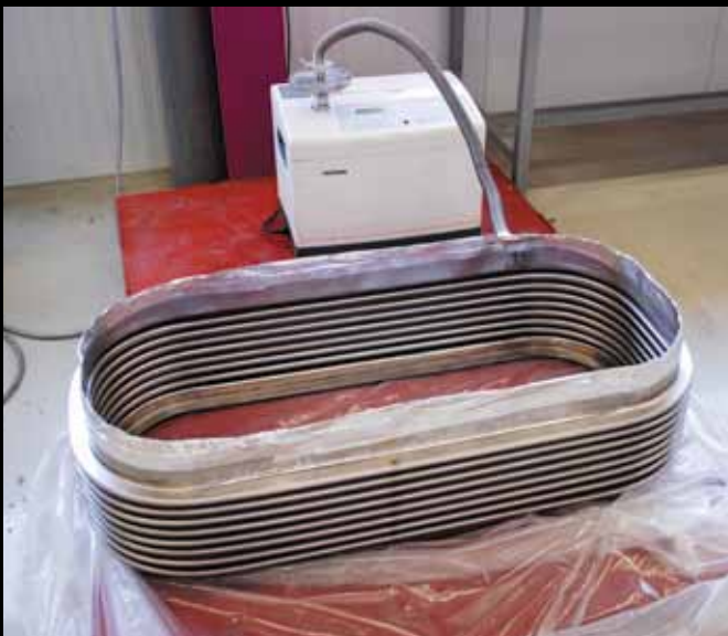
Helium leakage testing in the kompaflex own clean room
