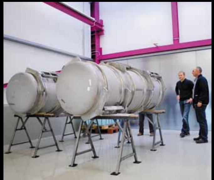
Water pressure test of expansion joints for a Nuclear Plant
